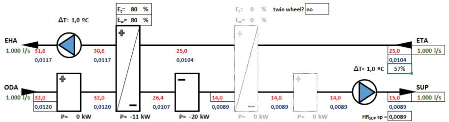
dry bulb temperature (°C) humidity ratio (kg/kg)
