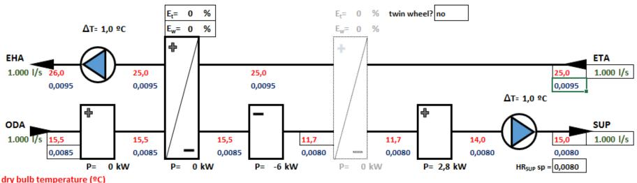
dry bulb temperature (°C) humidity ratio (kg/kg)
