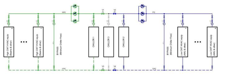
Redundancy can be created by hydraulically connecting both systems. A redundant chiller for both systems can be installed.
