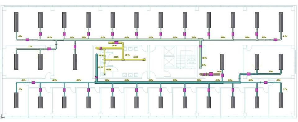
Duct is iteratively sized in order to optimize static pressure equalization between all duct branches to the beams.
