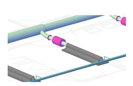
In this solution the beams are selected for the high density loads. Low density loads are managed by blanking beam nozzles.
