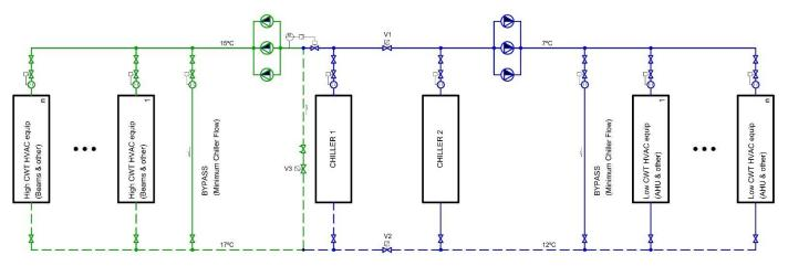
In case of faillure of one chiller the operating chiller produces water at 7°C and the beam water circuit operates in the mixing mode.
