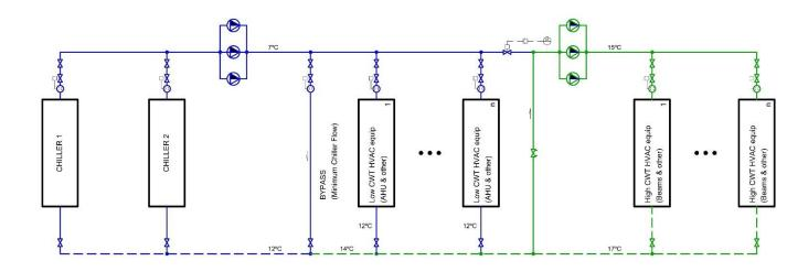
Most common beam water system. Chillers produce 7°C chilled water. Beam water circuit uses a mixing system.
