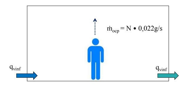
$$\dot{m}_{inf} = q_{vinf} \bullet \rho \bullet (HR_{ODA} - HR_{IDA})$$
