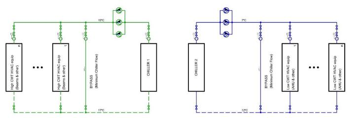
**Best efficiency solution.** Beam system is served by dedicated Chillers producing 15°C coolled water. Simple and reliable solution.
