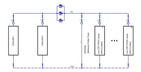
Most common system, operating with chilled water leaving ar 7°C and,(hopeffully) returning at 12.°C. Usually return water temperatures are much lower than 12°C decreasing chiller efficiency.
