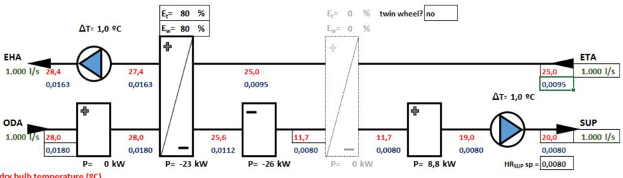
dry bulb temperature (°C) humidity ratio (kg/kg)
