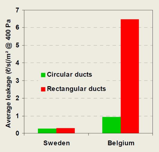
In Belgium, where there are no regulatory requirements for ductwork thightness, neither mandatory leakage testing, square section ductwork have a very high lekage rate.
